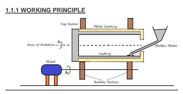
In this process a molten metal is poured into the spinning mould preheated to a certain temperature. The mould is placed vertically or horizontally based on the required shape of product. Once poured it is then continued to rotate about its central axis. Due to rotational motion of the mould, a centrifugal force is acted upon the molten metal just poured into the spinning mould. This force displaces the molten metals towards the periphery forcing them to deposit on the walls.
